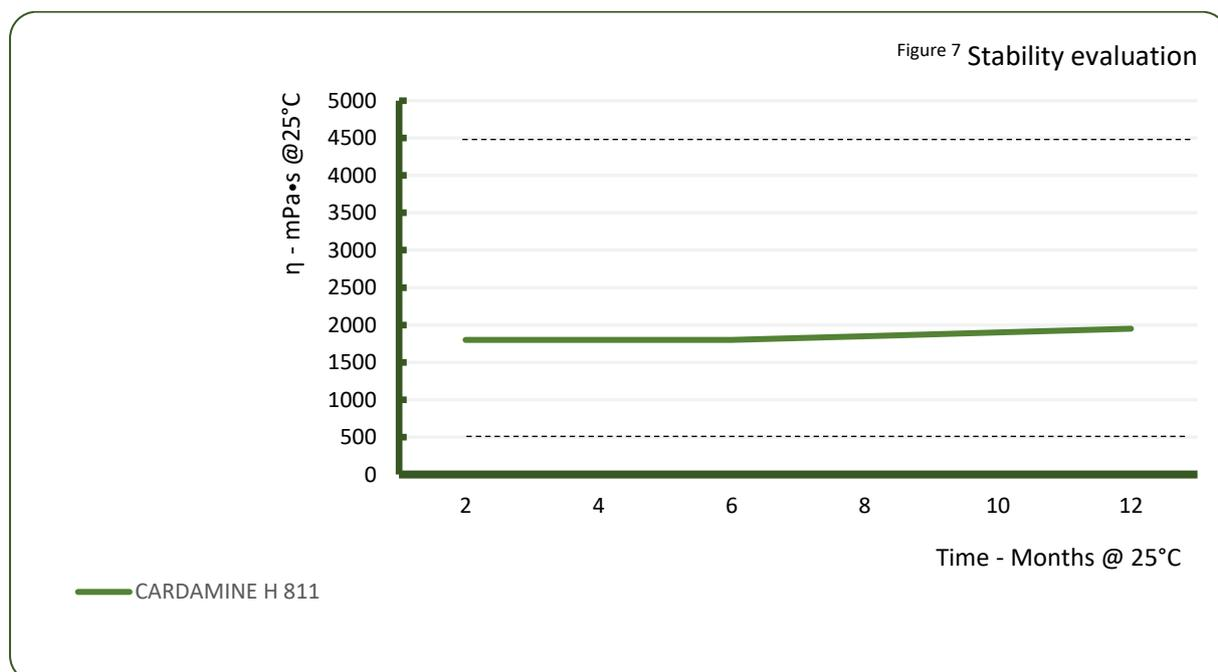
Viscosity conducted with a Brookfield viscometer @ 25C [ASTM D2556-14] and the material stored in sealed containers @ 25°C. In the case of the reactivity following storage, there was no appreciable difference.
