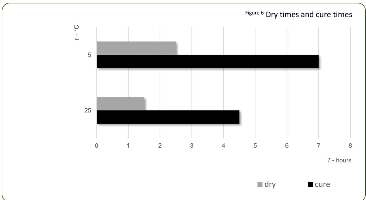
The graph above depicts the thin film reactivity at the temperatures indicated in the chart. Evaluation has been undertaken in combination with a stoichiometric quantity of EPILOK 60-600 [Bitrez Ltd], a liquid epoxy resin with EEW ≈ 190.
